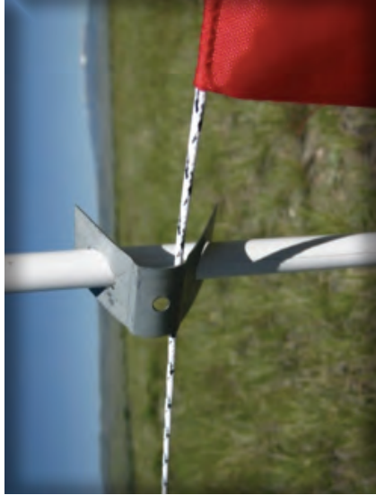
Figure 10: Galvanized clip for half-inch fladry posts; this clip is very strong.
